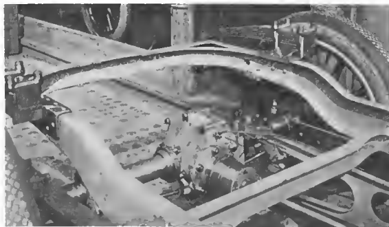
A Characteristic Drop Frame.
